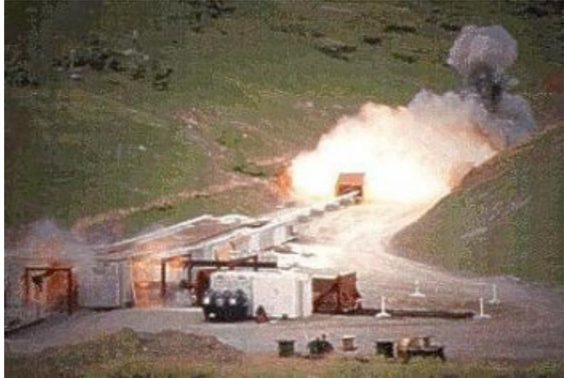
gas gun, a combustible gas (such as methane) first drives a piston in a cylinder that compresses a light gas (such as hydrogen). At a certain pressure, a valve ruptures to let the now very high pressure hydrogen into the second stage, smaller diameter barrel of the gun, accelerating the projectile.
