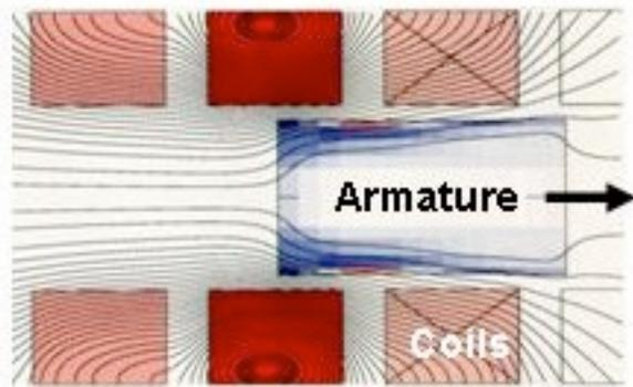
At Sandia National Labs, under the direction of Bill Cowan, several launchers were constructed. The first launchers had an unusual design that uses the main field of solenoidal coils rather than the fringing field. The projectile is a flat plate, which fits between two similarly-sensed drive coils. As the plate reaches the drive coils, current is switched on in
