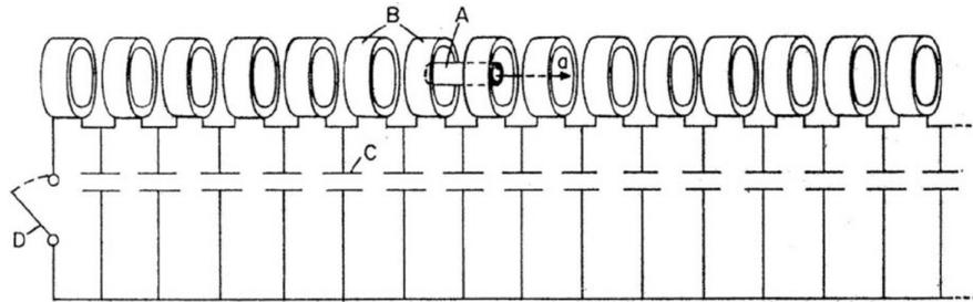
The driving coils in the Winterberg design are powered by capacitors, one capacitor per drive coil. For properly selected component values, the capacitors and coils act as a transmission line. Synchronization of the projectile with barrel is not necessary; other than the single initial switch, operation is passive. Unfortunately, no device based on this idea has been built. However, the term "collapsing field," which was to reappear at the University of Texas in 1993, was used by Winterberg.
